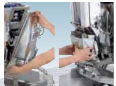
Unitization of actuator and feeder Easily removable and attachable buckets
