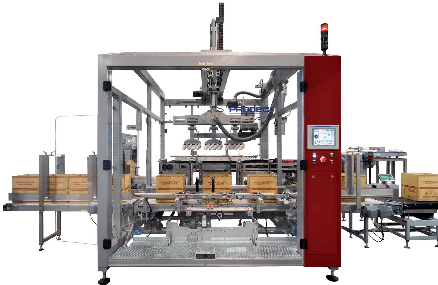
The **D-600** is a top packer with Pick & Place Cartesian system consisting of multiple case filling stations. The filling of cases is performed by a pick & place mechanism, with double leads, which supports several heads with speed which is adjustable according to product type. The system is expandable, depending on the required production output
