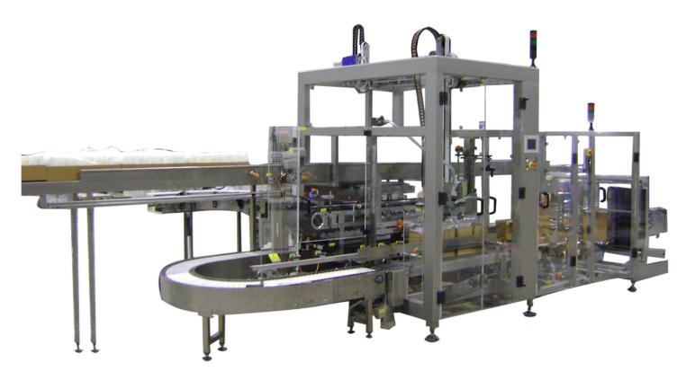
The **D-500** is a Pick & Place top packer consisting of multiple case filling stations. It also has integrated case forming, designed for medium and low capacities. The filling of cases is performed by a pick & place mechanism which supports several heads with speed which is adjustable according to product type. The system is expandable, depending on the required production output.
