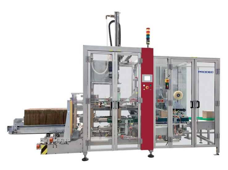
Superior solution for packing systems using Pick & Place multiple case filling stations in a single monoblock. With integrated forming and sealing of cases, designed specifically for small spaces. The filling of cases is performed by a pick & place mechanism which supports several heads with speed which is adjustable according to product type. The system is expandable, depending on the required production output.
