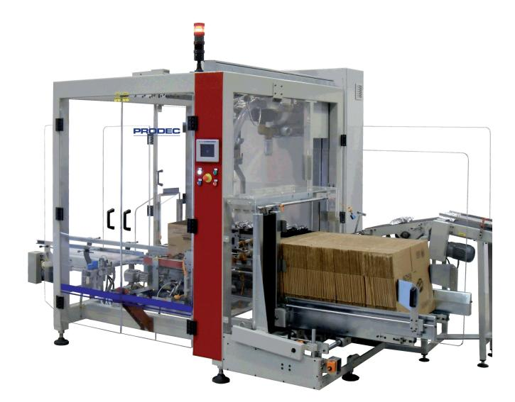
The **D-200** is a Pick & Place top packer with integrated case former, designed for medium and low capacities. The filling of cases is performed by a pick & place mechanism which supports several heads with speed which is adjustable according to product type. The system is expandable, depending on the required production output.
