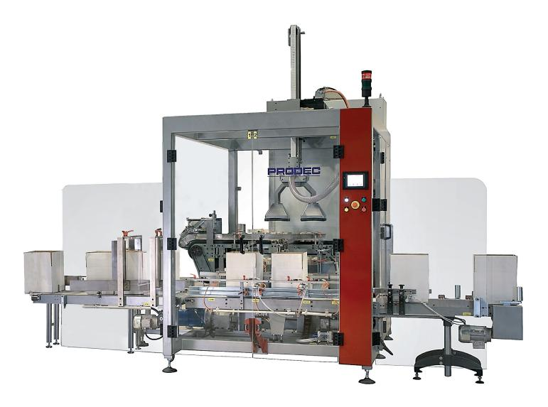
The **D-100** is a top packer with Pick & Place Cartesian system consisting of multiple case filling stations. The filling of cases is performed by a pick & place mechanism which supports several heads with speed which is adjustable according to product type. The system is expandable, depending on the required production output.
