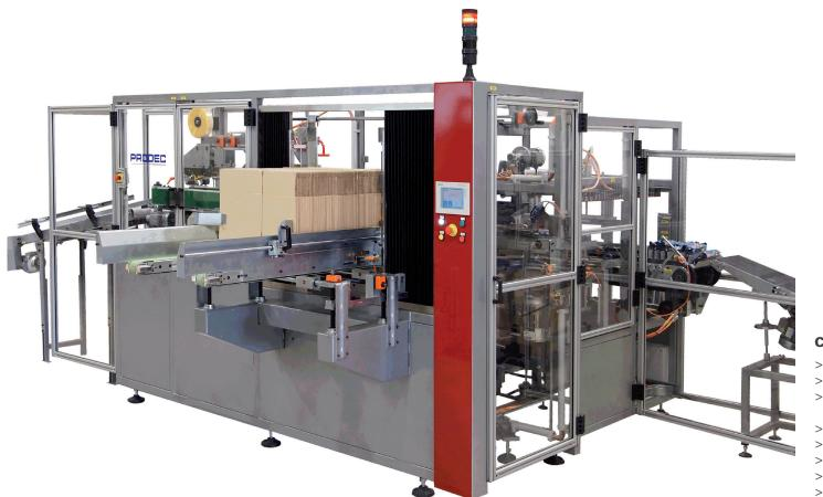
The **FI-1** is bottom loading, modular, compact and flexible case packer, designed for medium per minute case production, all in a single monoblock.
