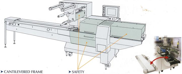
Easy cleaning cantilevered frame design allows product crumbs to fall through the wrapper. Hygienic stainless steel covers are standard. Also, the height of the frame is 165mm from floor in order Safeness of control system related to safety such as cover safety and emergency stop are designed based on Category 3.
