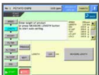
Automatic program setting display
