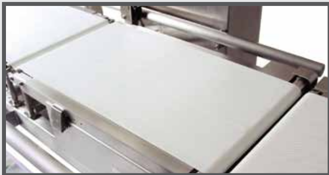
Anti-bacterial conveyor belt
