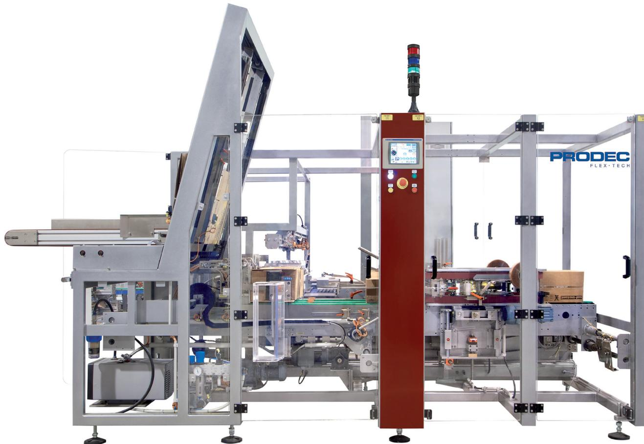
The **FL-5** is a side loading, modular, compact and flexible case packer, designed for medium per minute case production, all in a single monoblock.
